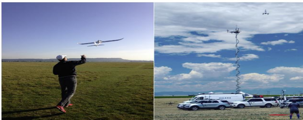
Fig 1- Hand-launched unmanned aircraft systems (UASs) can be used to collect and monitor plant pathogens in the atmosphere (left). Rotary-wing UASs equipped with weather and particle monitors can be used to collect weather and pathogen data (right)
